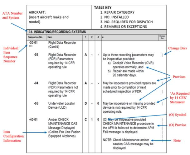
Figure 3-1. Example MMEL ATA Coded System Section Page
